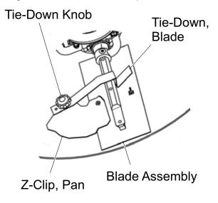
Figure 45. Z-Clip Finisher Pan Installation
